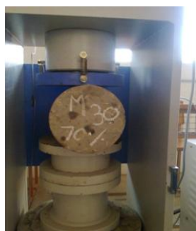
Figure. 5.2 Split Tensile Test
